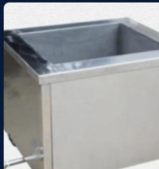
Other brand cleaning machine flat cylinder mouth, water is easy to splash out
